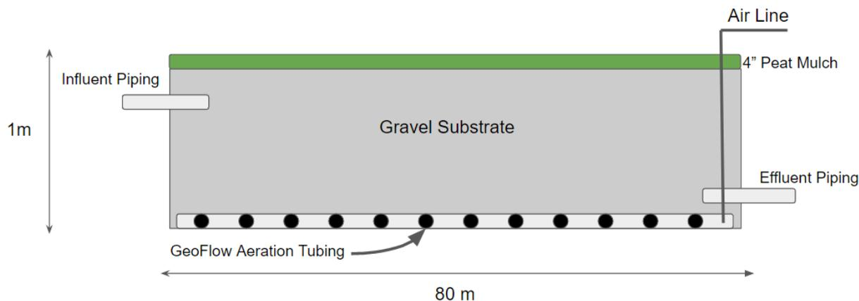
**Figure 6.3.** Schematic of a subterranean aerated gravel bed (adapted from Nivala et al. 2013) [22].
