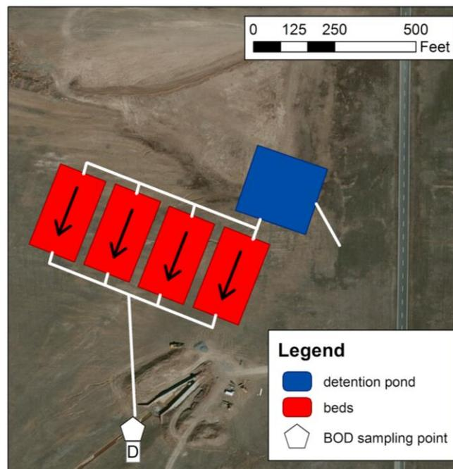
**Figure 6.2.** Plan view of proposed layout for subterranean aerated gravel beds and corresponding detention pond near sampling location D.
