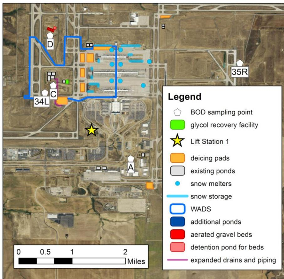
**Figure 4.1.** Map of deicing infrastructure at DIA and locations of proposed alternatives.
