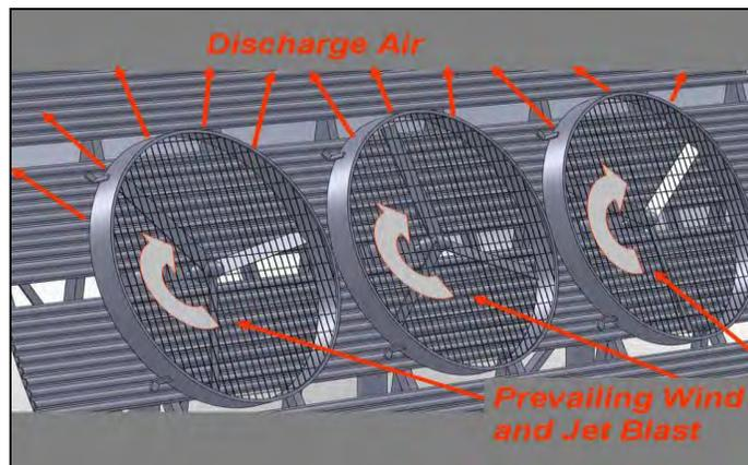
**Figure 1-1 Wind-Flow Patterns through AfWATT**
