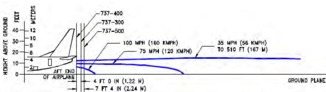
**Figure 5-4 Boeing 737 Breakaway Thrust Jet Blast Speeds**
