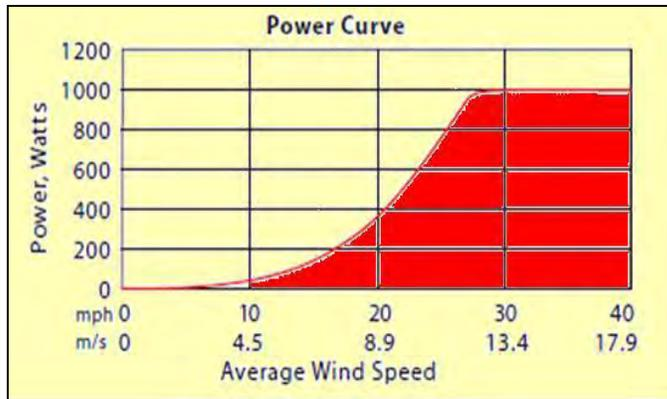
**Figure 2-2 Wind Speed Power Curve**
