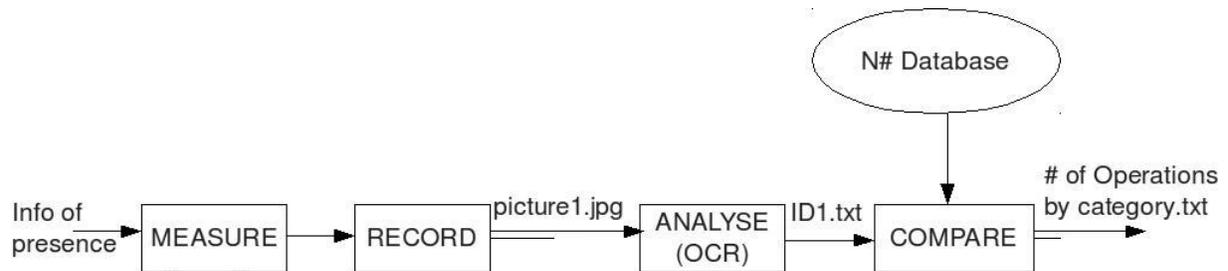
Figure 4: System Overview Schematic
