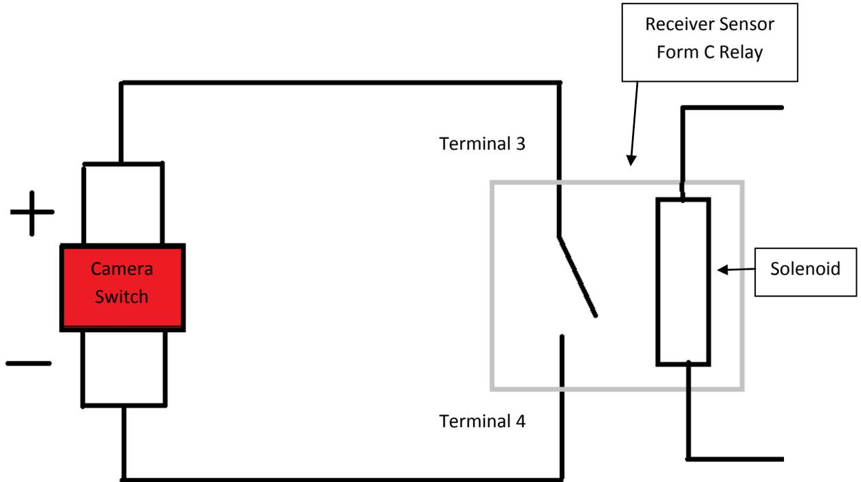
Figure 14: Camera Wiring Schematic
