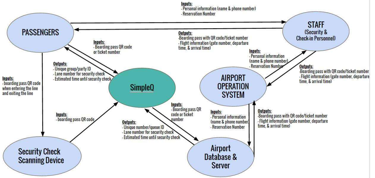
Figure 5.5: Component Interactions with SimpleQ System
