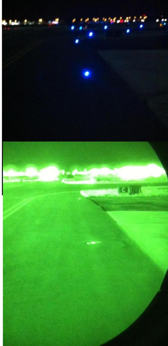
*Figure 7.5. LED taxiway lights rendered invisible by NVGs*
