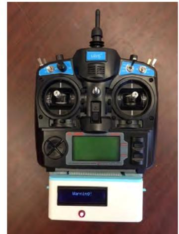
Figure 13: Drone Operator Notification System receiver housing with components attached to drone remote control.
