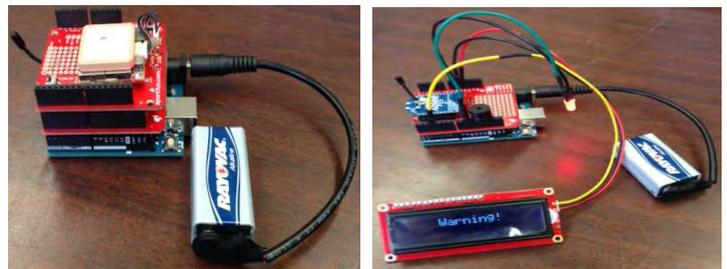
Figure 14: Drone Operator Notification System transmitter subsystem (left), receiver subsystem (right).
